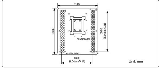
Figure 2 External dimensions of the PCA7752AG02
